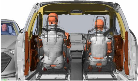
Fig.4 Car to car simulation to select test condition (occupant movement)
